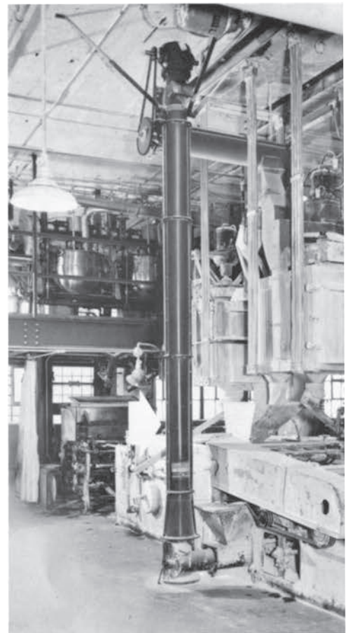
Candy manufacturer employs Screw-Lift in ingredient distribution system.
