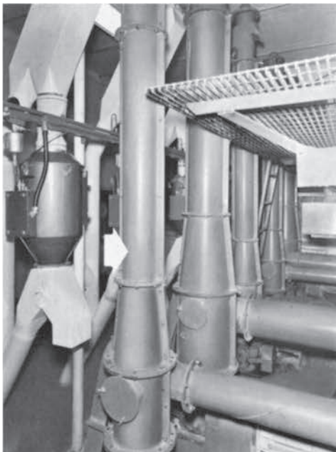
Multiple installation shows compact arrangement possible with the Screw-Lift.
