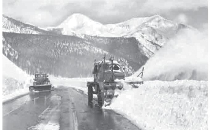
Special flighting provides fast, clean snow removal. This type of flighting has been used since 1932.
