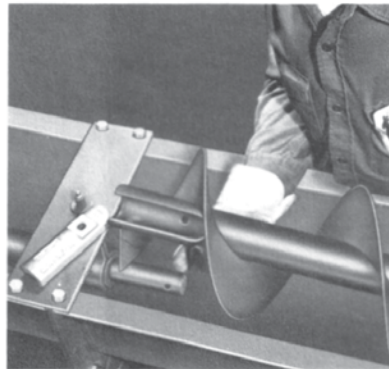
Lift the conveyor section out and perform necessary replacement or repairs.
