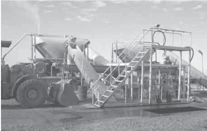
Screw Conveyors are used to convey multiple materials including wet and dry. This installation demonstrates how liquid material can be conveyed up an incline for ease of loading trucks. All parts of the system are enclosed yet readily accessible.
